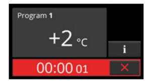
Upon completion of the thaw program, the end of cycle (EoC) alarm will sound. The controller will automatically revert to "hold" mode.
