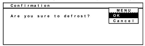
**3.** The manual defrost is started. During defrosting, "Defrosting" is displayed at the upper left on the top screen.
