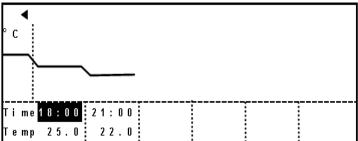
Change the step number and cycle number to 2Stp and 99Cyc by character input key. Only one page is displayed and 99 is changed into  $\infty$ . Display of  $\infty$  changes to 99 when placing a cursor.
