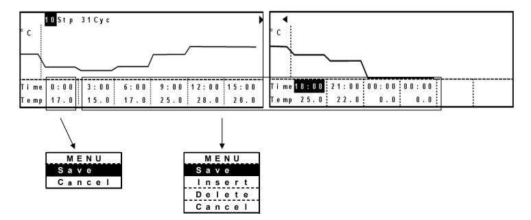
The step number (Stp) can also be changed by "Insert" or "Delete" on the menu window. Press the menu button (MENU), to open the menu window. The menu window for a first section has no "Insert" or "Delete". Therefore, neither insert nor delete is effective for the first section. The maximum step number is 12. The cycle number is 1 when the step number is 1. The settable cycle number is up to 98. The cycle number 99 means limitless repeat.
