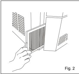
**3.** Clean the filter by a vacuum cleaner and replace to the original position.
