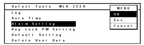
**2.** The Alarm Setting screen is displayed. On this screen, the automatic set temperature alarm (Temp Alarm), the automatic set humidity alarm (RH Alarm) (For MLR-352, it is not possible to set), the automatic set temperature alarm delay time (Alarm Delay), alarm resume time (Ring Back), the door alarm delay time (Door Alarm Delay) and door alarm resume time (Door Ring Back) can be set.
