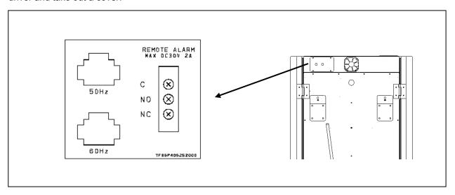
The remote alarm terminal is a contact output. Contact capacity is or 2 A (DC 30 V).
