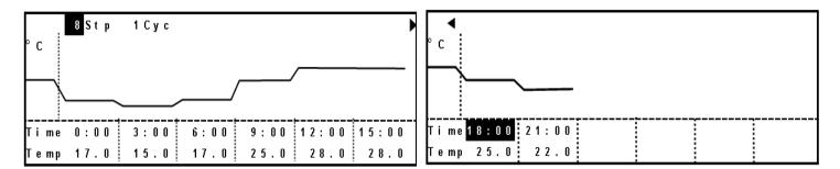
The step number (Stp :step) and cycle number (Cyc :repeat number) can be changed on the top left corner (8 Stp 1 Cyc) of the screen. Highlight the numerical value by shift key, and input 10 Stp 31 Cyc by character input key. The step number and cycle number are changed.
