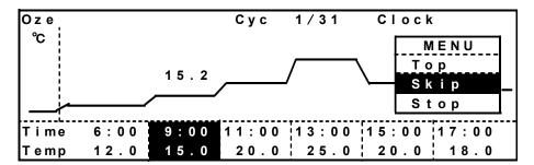
**3.** The Confirmation screen is displayed. Press the menu button (MENU). Selecting "Next" causes the skip to the next step. Selecting "Back" causes the skip to the previous step. After selecting "Next" or "Back", press the enter key (ENTER).
