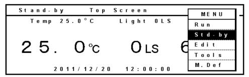
**2.** Stand-by Setting screen is displayed. Set each parameter. Press the menu button (MENU) after complete parameter setting. The menu window is shown. Select "OK" and press the enter key (ENTER). The parameter is memorized.
