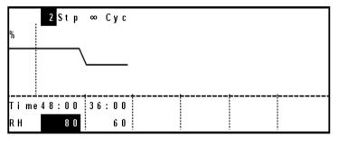
**Note:** The time setting value differs between clock mode and timer mode. In the case of timer mode, setting range is between 00:01 and 99:59. The setting of "99:99" means limitless repeat.
