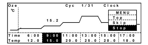
**3.** The Confirmation screen is displayed. Selecting "OK" and press the enter key (ENTER) to stop the program.
