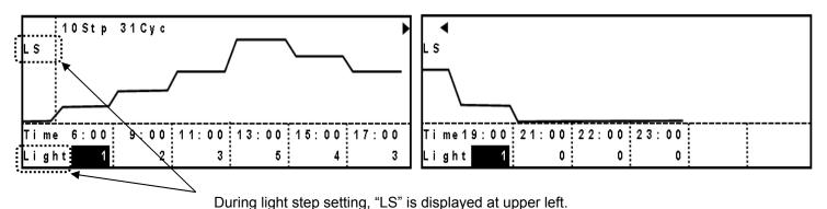
**8.** For MLR-352H, shifting a cursor downward further by the downward shift key moves to the next edit "RH" (relative humidity). For MLR-352, shifting moves to the edit "Temp".
