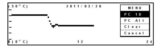
**2.** The Progress screen is displayed. Specify a transfer, capture of text and retention file by operation of hyper terminal on PC. Apply "txt" or "csv" as an extension of retention file. Press the menu button (MENU) to show the menu window. Select "Start", and press the enter key (ENTER). The transmission is started. "Finished" display means the end of transmission.
