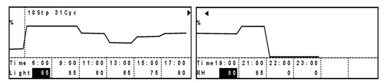
Set a relative humidity as below. The setting range is between 55 %R.H. and 90 %R.H. (Input range : between 50 %R.H. and 90 %R.H.).
