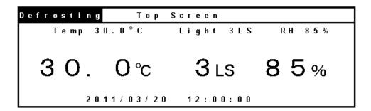
**4.** The manual defrost is finished automatically. The defrosting time depends on the amount of frost on the evaporator.
