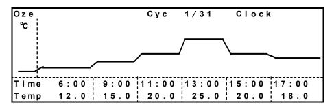
**5.** The program is started at desired date and time. During the programmed running, the graphic screen as below is displayed. To change the graphic screen to the top screen, press the menu button (MENU) to show the menu window. Select "Top" and press the enter key (ENTER). To change to the graphic screen, press the menu button (MENU) to show the menu window. Select "Graph" and press the enter key (ENTER).
