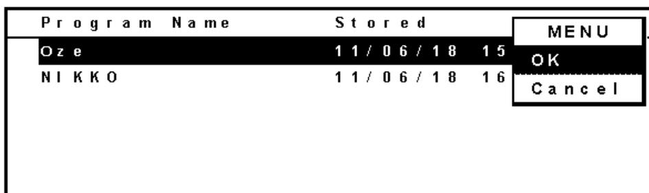
3. Start Options screen is opened. On this screen, setting of Timer (selection of Clock mode or Timer mode), Join (Joining some programs), and start date is available. As the "Oze" is for clock mode, select 1 (Clock) for Timer. For join, select 2 (No : not join) since the Oze does not have joined program. Input the start date (11/12/20) and time (06:00:00), and press the menu button (MENU) to show the menu window. Select "OK", and press the enter key (ENTER).
