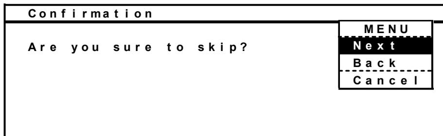
**Note:** It cannot go back prior to the current time by the skip function when the program is running in clock mode.
