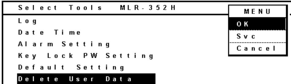
2. The Delete User Data screen is displayed. To select a program to be deleted, select "Delete a User Program" and press the menu button (MENU) to show the menu window. Select "OK" and press the enter key (ENTER).
