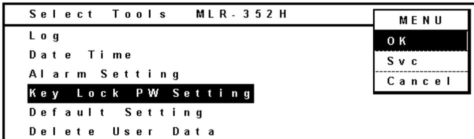
2. Input the Current User Password (4 digits). Press the enter key (ENTER). The default User Password when shipped from the factory is "0000".
