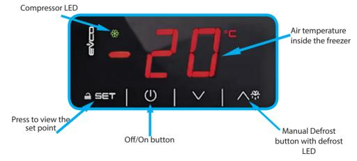
Your freezer is preset to  $-20^{\circ}$ C so you do not have to program the set point. To check the set point, simply press the  $\triangle SET$  button.
