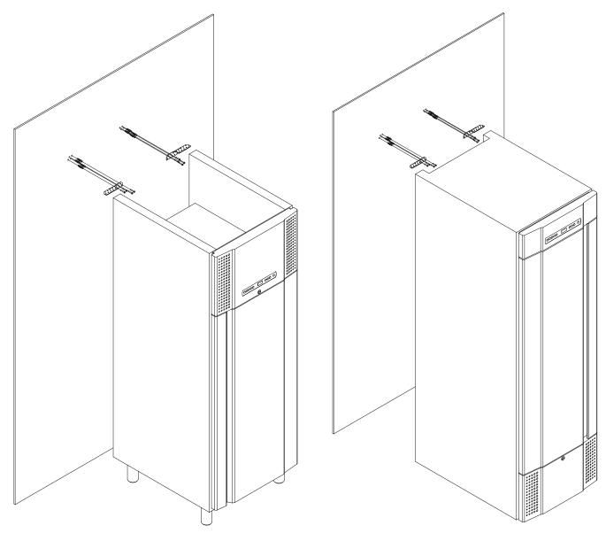
The tilt brackets must be fitted when installing the cabinet, ensuring that the users, surroundings and stored items are not damaged by the cabinet.
