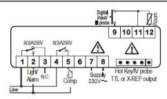
9-40Vdc supply: connect to the terminals 7 and 8. 12Vac/dc supply: connect to the terminals 7 and 8. 24Vac/dc supply: connect to the terminals 7 and 8. 120Vac supply: connect to the terminals 7 and 8.
