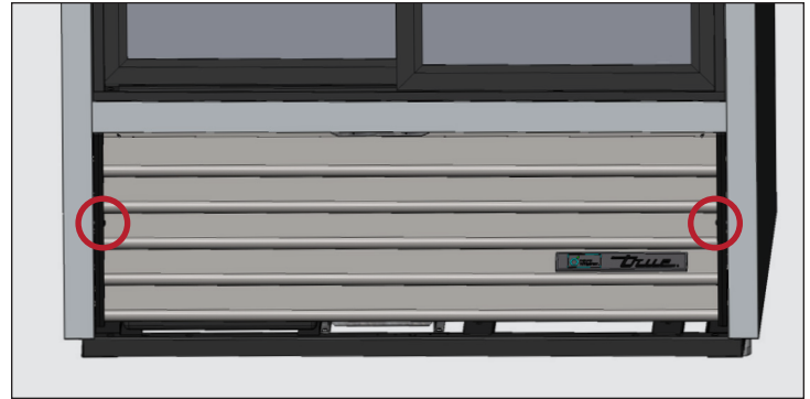
Fig. 2. Slide door louver grill screw locations.
