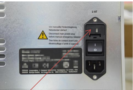
Fuse drawer with fuse 4 AT
