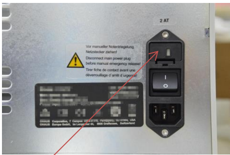
Fuse drawer with fuse 4 AT
