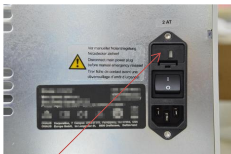
Fuse drawer with fuse 4 AT
