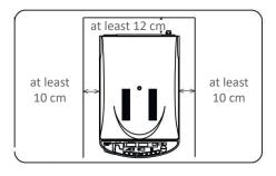
Please place the unit at least 10 cm from the side and at least 12 cm from the wall at the rear. Please note that the unit should not be installed in places where the room temperature is below 5 °C or above 35 °C.
