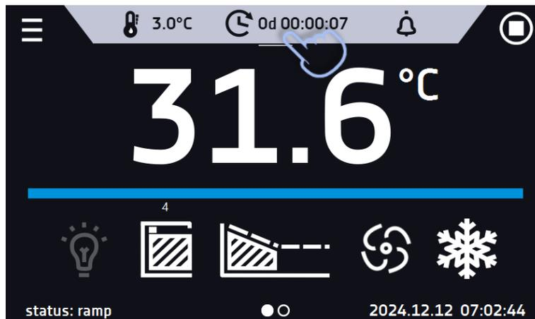
Figure 40 Quick change of set time - value setting
