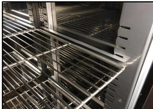
To remove a shelf, perform the above steps in reverse order. To remove the shelf slide from the slots, lift it up and slide it towards the rear of the chamber.
