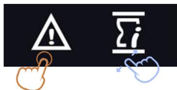
In the alarms panel there's a list with active alarms or the alarms that have occurred but have not been confirmed. When the alarm is active, the alarm bar is red and the alarm event is displayed in the list with the status "active". When the alarm event stops, the state changes to "inactive".
