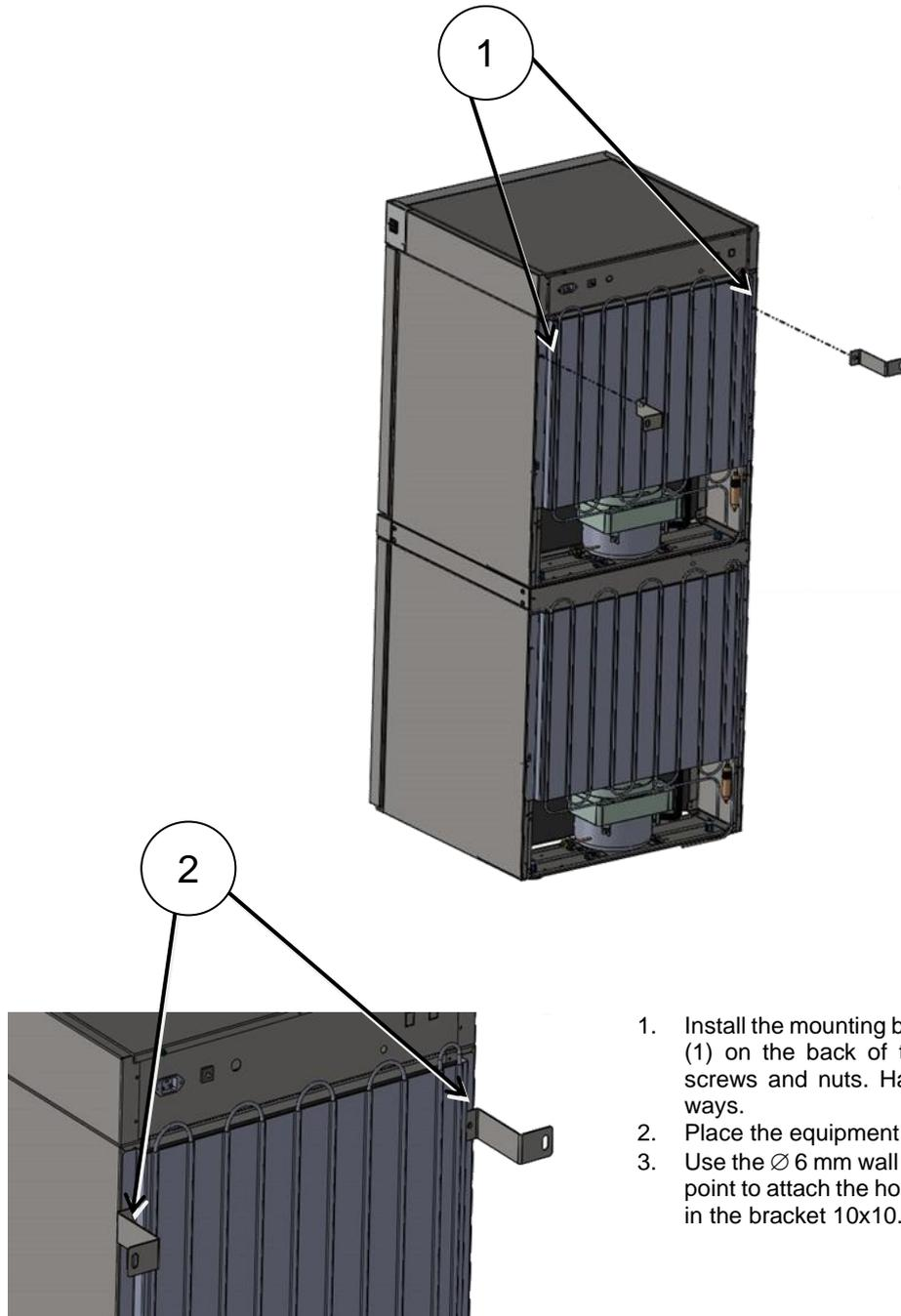
1. Install the mounting brackets (2) to the holes marked (1) on the back of the device using the supplied screws and nuts. Handles can be set up or sideways.
