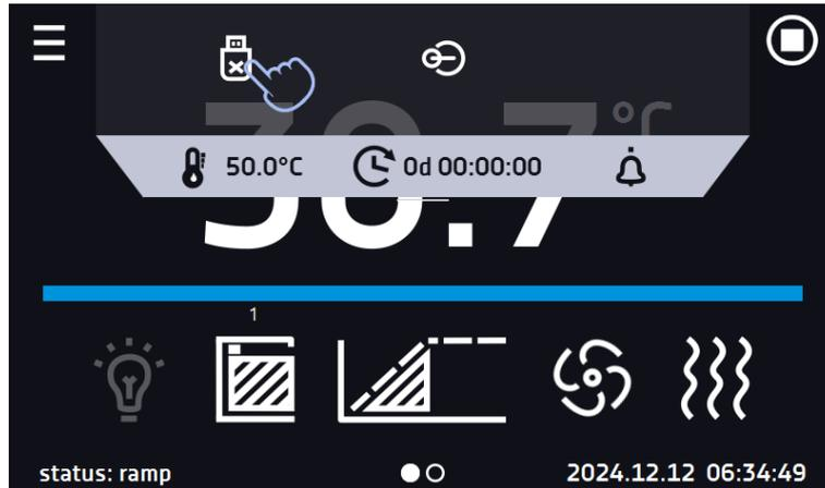
Data saved in the \*.csv file can be opened in a spreadsheet. Data saved as \*.plx can be opened in the Lab Desk program (additionally paid option). This program allows, among others, for data preview in the form of a table or a graph. It also allows you to prepare a statistic report for a selected range of data, see [Section 6.1](#).
