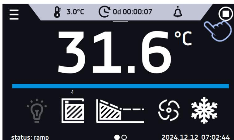
Figure 42 Quick change of fan efficiency- value setting
