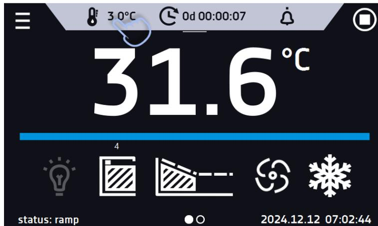
Figure 38 Quick change of set temperature - value setting
