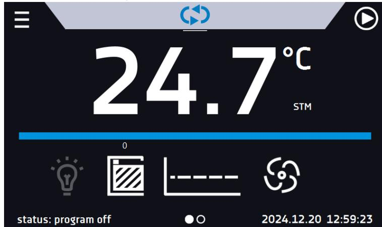
Figure 61. STM Function - option enabled, program running
