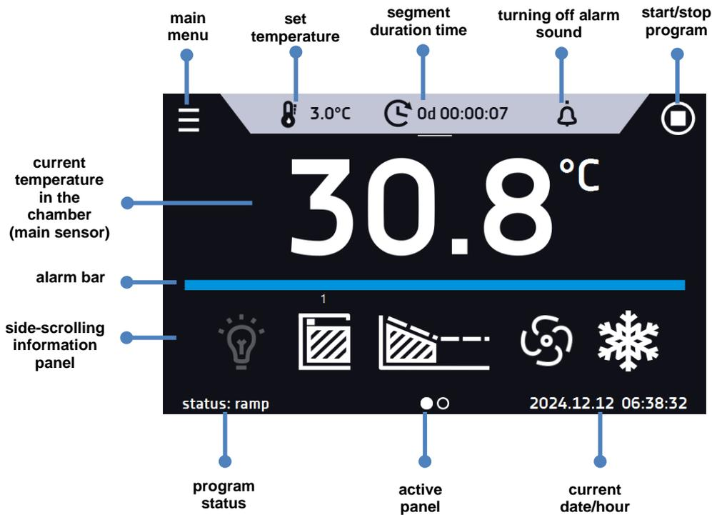
Figure 10. Main screen – running program in ILW
