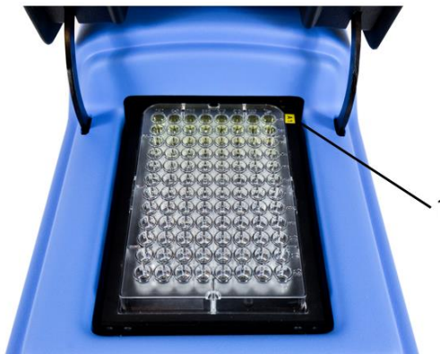
Figure 3. Correct microplate placement.
