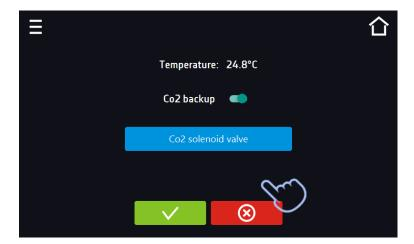
When the button is pressed, the CO2 valve opens, accompanied by a loud noise and a drop in temperature.
