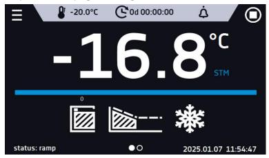
Figure 55. STM Function - option enabled, warning about problems with achieving/maintaining temperature.
