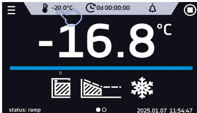
Figure 33 Quick change of set temperature - value setting
