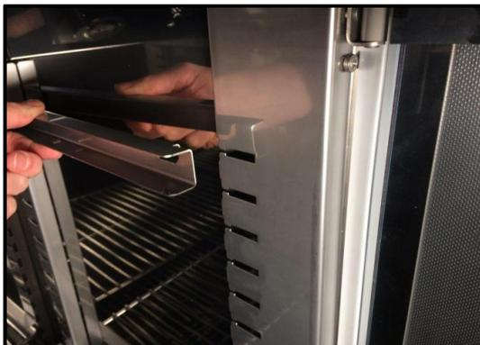
Slide the shelf into the installed shelf slides. Now, the shelf is correctly installed!
