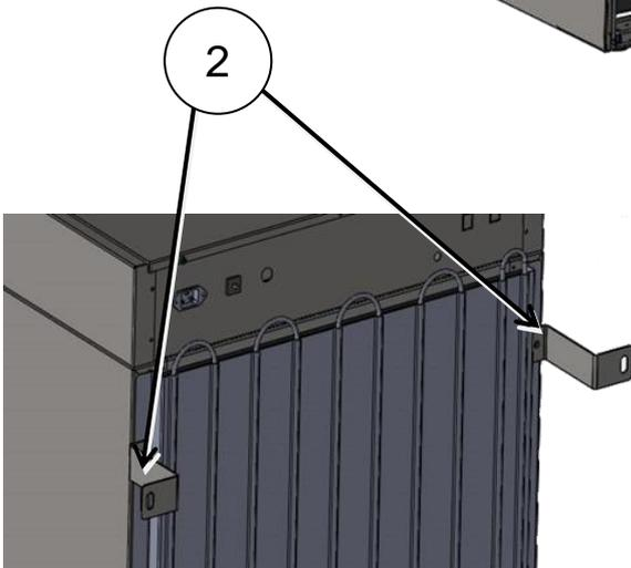
1. Install the mounting brackets (2) to the holes marked (1) on the back of the device using the supplied screws and nuts. Handles can be set up or side-ways.
