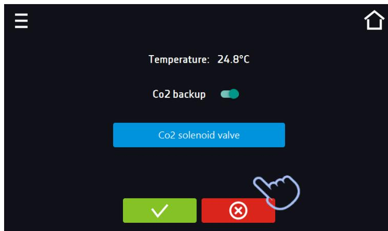
When the button is pressed, the CO<sub>2</sub> valve opens, accompanied by a loud noise and a drop in temperature.
