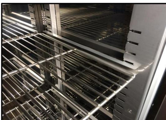
To remove a shelf, perform the above steps in reverse order. To remove the shelf slide from the slots, lift it up and slide it towards the rear of the chamber.
