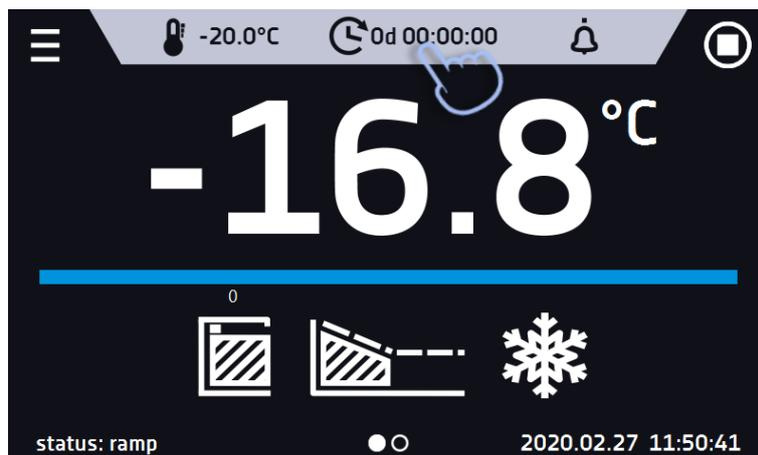
Figure 35 Quick change of set time - value setting
