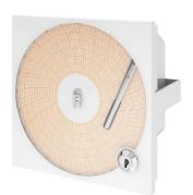
The equipment are designed to accommodate a circular chart recorder.
