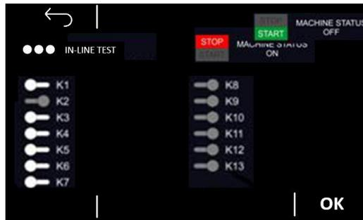
With the temperature regulation in progress, the upper right part of the screen allows you to lock or distribute the temperature control of the equipment to be able to take the manual control.
