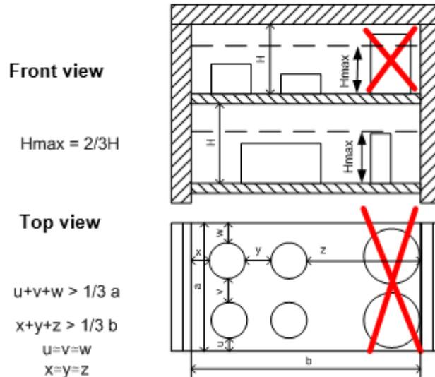
Following the above recommendations will ensure the most optimal temperature stability and uniformity
