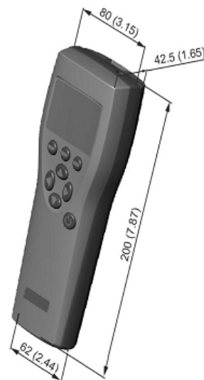
MI70 indicator dimensions in millimeters (inches)
