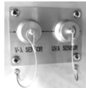
Figure 14: Connection sockets closed with protecting caps
