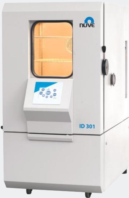
*ID 301 Climatic Test Cabinet is designed to simulate natural climatic conditions. By means of the wide range of temperature and humidity control of ID 301, various kinds of products can be tested at different climatic conditions and stability, artificial aging and storage tests can be easily done as well. The reliability, performance, operability and safety makes ID 301 one of the indispensable equipment for quality control and R&D in:*
