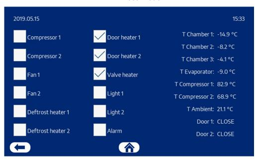
Test Mode for when the unit is switched ON.
