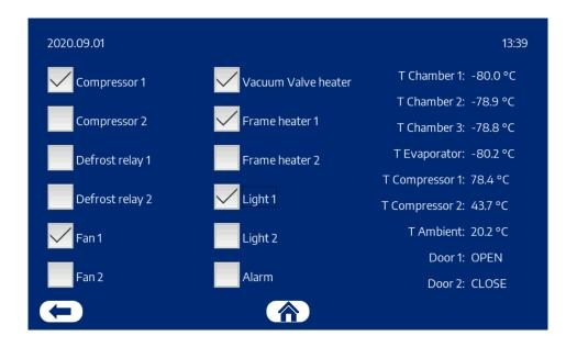
This feature is for service and maintenance use. By this Test mode, you can check all relays and door contacts and check the temperature sensors.
