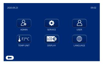
Type in the pin code for Service level, and push the OK button.
