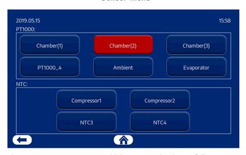
When a Sensor alarm occur, you can see which one are having a failure. Click on the red button to deactivate the alarm.
