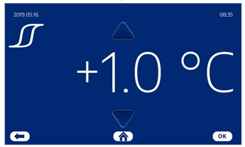
Hysteresis settings: The temperature between start and stop of the Compressor.
