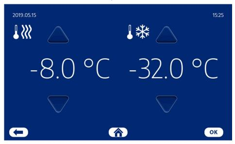
To set up the High and Low temperature alarm.
