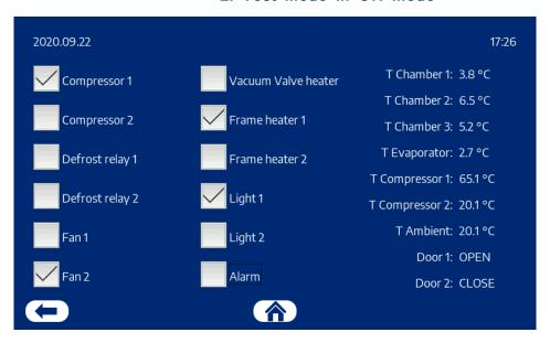
When the unit is Switched ON and running, you can see: Which relays are ON or OFF, the temperature of each sensor, and position of Door contact.
