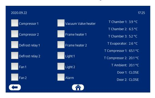
When the unit is OFF, you can simulate each relay by pushing the square field, for testing each kind of device. (Compressor, Light, Fan motor etc.) Very good feature for service and maintenance use.
