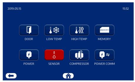
Under alarm list it is showed which type of alarm that are occurring. The Button will be red when the failure is activated, and the remote alarm relay will be active until you click on the red button to deactivate the alarm.
