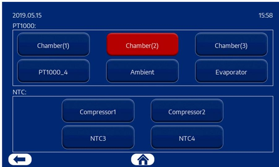
When a Sensor alarm occur, you can see which one are having a failure. Click on the red button to deactivate the alarm.
