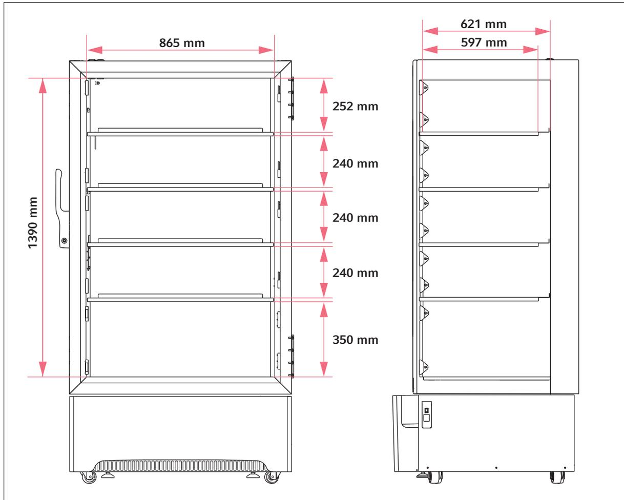
Fig. 10-1: Internal dimensions for devices with 5 inner compartments
