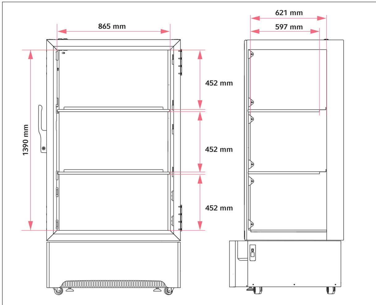
Fig. 10-2: Internal dimensions for devices with 3 inner compartments
