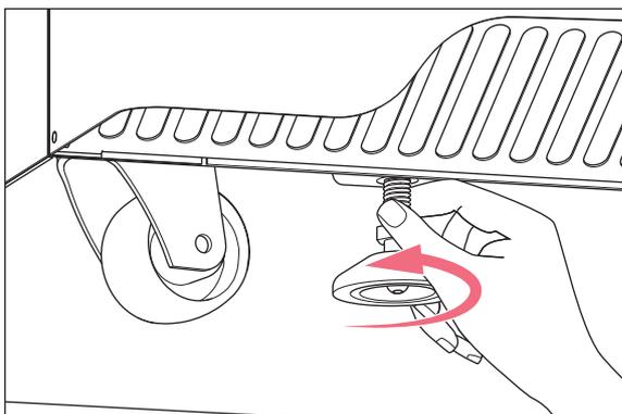
2. Rotate the leveling feet down.
