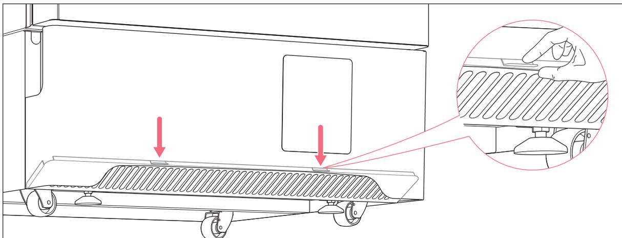
Fig. 7-1: Folding down the air intake grille
