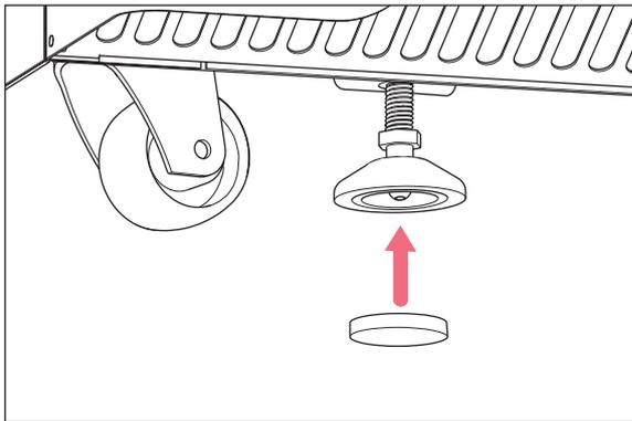
1. Attach anti-slipping pads to the underside of the leveling feet.
