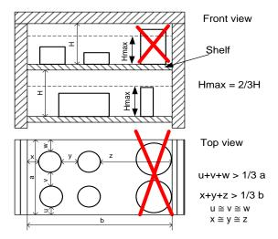
Following the above rules will provide best optimal parameters of temperature fluctuation and variation.
