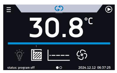
Figure 9. Main screen - running program in ST, CHL
