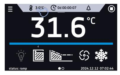
Figure 38 Quick change of set temperature - value setting
