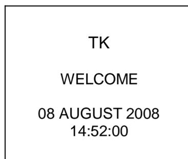
After 5 seconds the LCD display goes to stand-by position with a short signal.
