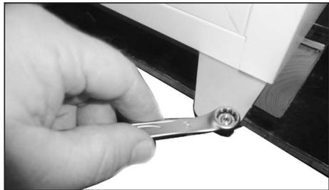
24. Remount and tighten pivot nut
