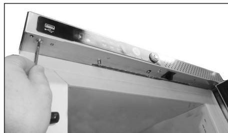
4. Remove three screws underneath the toppanel (use 3 mm allen key)
