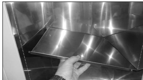
Lift up to release all hooks and pull the shelf to one side. Then tilt the shelf upwards in the free side and lift it out
