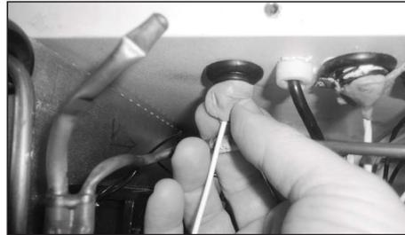
9. Closed the port hole by using putty
