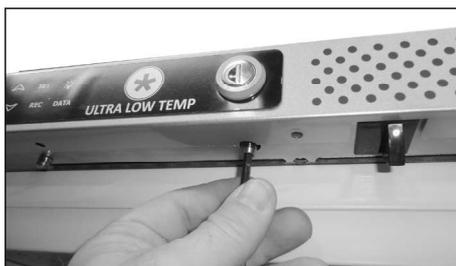
5. Remove lock pin (use 4 mm allen key)
