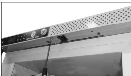
41. Remount the three screws upwards in the toppanel...
