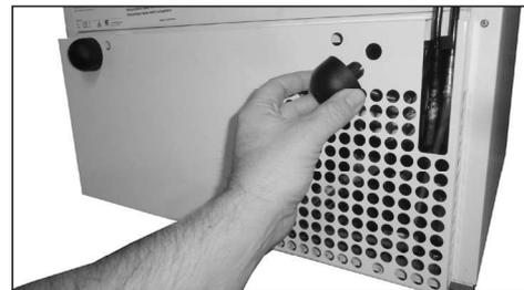
2. Then locate the identical hole in the right side of the engine cover and push the last guard into this hole
