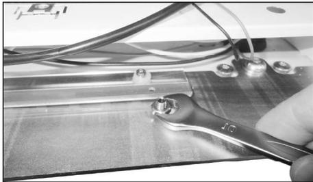
15. Demount fix nut and top handlelock pin
